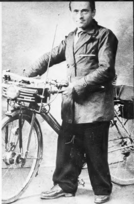
Radio-Bike: a bag in the rear holds the batteries for a four-tube radio. Paul Bayrad, a mechanic of Veray-Sur-L'ognan, France, is the owner-designer-builder of this 56-pound motor bike which allows him to listen to favorite programs.
